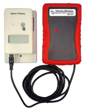
Tehama's Bluetooth Display Programmer gives field technicians the ability to program a Display MDT from Tehama Connect Mobile App (Android and iOS), avoiding the need to lug around a laptop. The Programmer runs on two AA batteries and is easy to use. Simply power on the Bluetooth Programmer, pair it to your smart phone from within the App, then plug the cable into the Display MDT.
