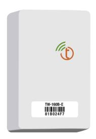
The Standard Range Encoder MDT has a true encoder interface that directly reads the meter face value of encoded meters to transmit an absolute reading towards the DCAP every hour. It auto-detects the data format between Sensus meters, Sensus compatible meters (Master-Meter, Badger, etc.), and Neptune meters.
