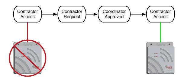
A field technician wanting access to a DCAP will make an Access Grant request for a specific DCAP using our CIT software or our Mobile App. Within seconds the coordinator, also using the CIT, will scan for new Access Grant requests and can approve it. Once it is approved, the field tech will be able to use the Grant to connect to the DCAP for the amount of time approved by the Coordinator.
