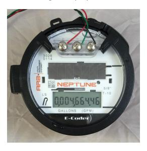
The picture here shows a 5/8" E-Coder register with nine digits total, two digits of which are to the right of the decimal (1/100 of a gallon resolution). But since only the upper six digits are available to the MDT, it will report 466. Apply a 10X count factor to get 4,660 gallons when displayed in the CIT or a daily report, even though the register shows 4,664.46 gallons.
