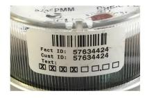
The meter above has eight rotating dials. However the factory sticker shown on the right says only 4 digits are available to an external reader. So the MDT in this case will report the value 7. Apply a 100X count factor to get 700 cubic feet, even though the register shows 729.62 cubic feet. Once the register shows 800.00, the MDT will report 8 (or 800 with the proper count factor applied).
