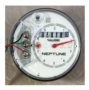
**However**, Neptune further reduces the effective count factor by *only* reporting a 0 or a 5 for the lowest moving dial. While the count factor is still 10 for this meter (because of the one fixed zero), any reader such as our MDT will only detect a change in reading every 50 gallons! For the larger meters with two fixed zeros the MDT can only detect a change every 500 gallons (and the count factor is 100).
