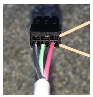
Insert small screwdriver into top hole to remove wire.
