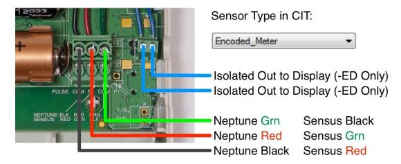
Our TW-140B-ED unit additionally provides a pulse output to drive a remote display as required in California. This output is an isolated dry-contact type and can drive any display that accepts this type of input. There is no polarity associated with this connection. The wiring colors for each meter type is written on the board to simplify installation.
