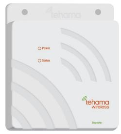
Our new MAX range Diversity RF Repeater receives radio messages from MAX series MDTs and Repeaters and then retransmits the message with its +28dBm high power radio toward the data collecting DCAP. Our Max Range products use Spread Spectrum technology to triple the range over our standard Range products. All Tehama Repeaters implement a redundant and self-healing 2-way mesh radio network between MDTs and the DCAP. MAX range products are not compatible with our Standard Range products.
